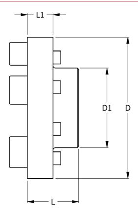
D = 480 D1 = 300 L = 190 L1 = 65 Max bore = 180 Torque (N m) = 16600
